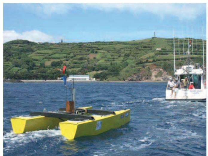
**DELFIMx and Águas Vivas performing a coordinated target tracking manoeuvre**
